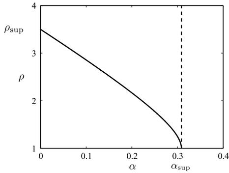
**Fig. 3.** The coarseness  $\rho$  of the logarithmic quantizer vs the loss probability  $\alpha$ . The dashed line is the upper limit  $\alpha_{\text{sup}} = 1/\prod_i |\lambda_i^u|^2 = 0.31$  of  $\alpha$ .
