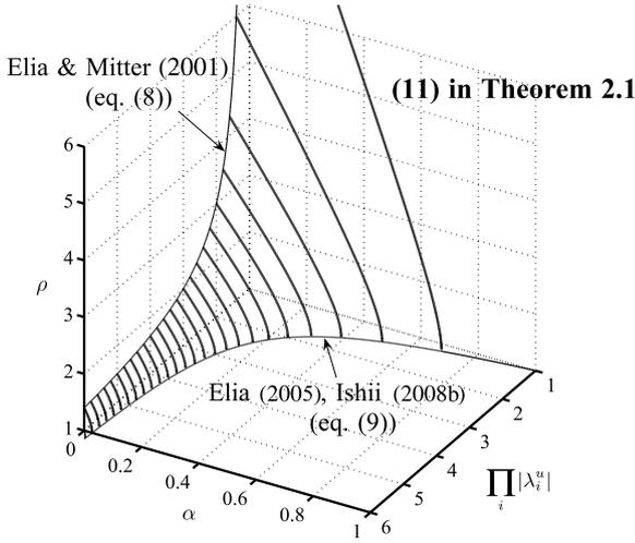
**Fig. 2.** The relationship between the product of unstable poles  $\prod_i |\lambda_i^u|$ , the loss probability  $\alpha$ , and the coarseness  $\rho$  of the quantizer.
